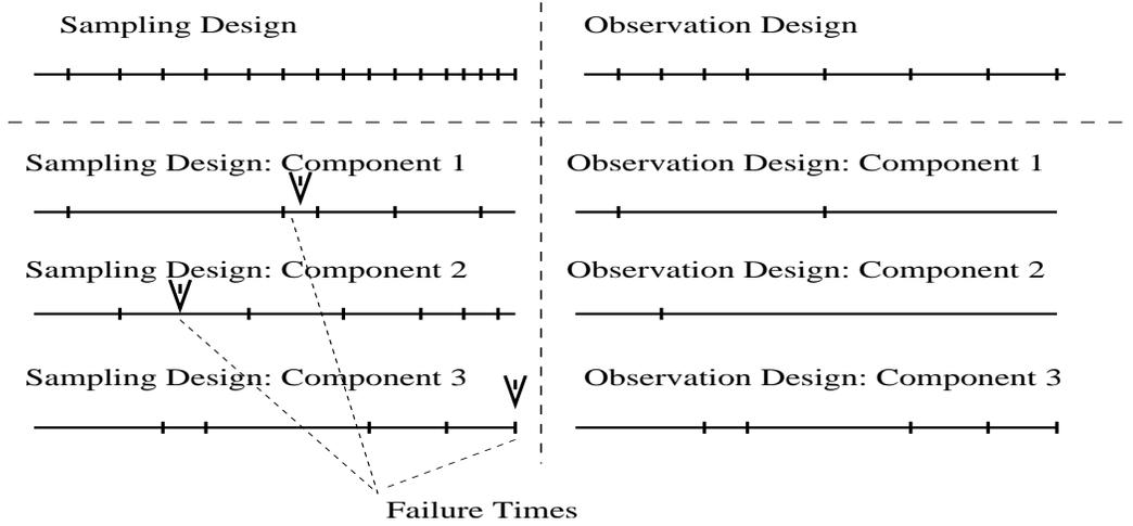
Fig 3: Non-uniform sampling: Sampling time points vs. observation time points.
